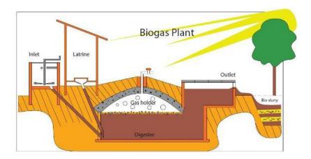
Bio-gas, in other words methane can be generated by anaerobic digestion with anaerobic bacteria or fermentation of biodegradable materials such as manure, sewage municipal waste, green waste, crops and plant materials, animal's excretion etc.
