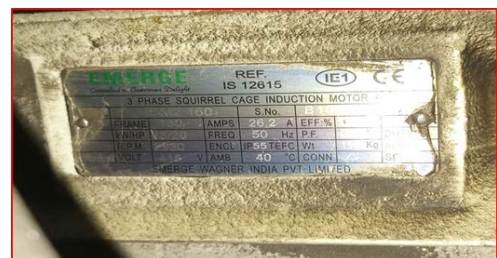
Name Plate Details of New EE Motor – 20 HP Emerge Wagner Make
