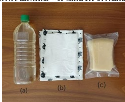
Plate 3.1 Materials used for preparing beeswax-coated cotton food wraps - (a) Coconut Oil, (b) Organic Cotton Fabric (125 GSM), (c) Pure Beeswax.
