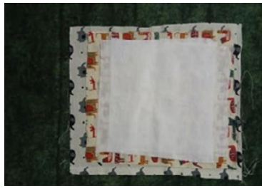
Plate 3.4 Cotton fabric cut into required sizes for coating.
