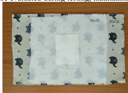
Plate 3.7 Inspection of coated cotton wraps for uniformity and even ness.
