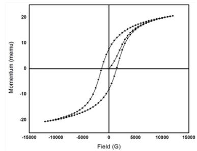
Figure 13 Hysteresis Loop of Lead Ferrite Synthesized by Sol Gel Method
