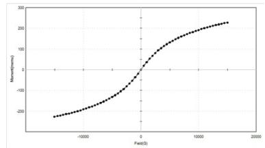
Figure 14 Hysteresis Loop of lead ferrite synthesized by hydrothermal method
