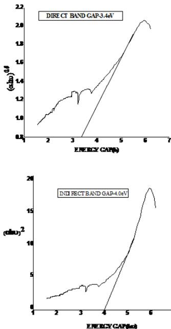
**Figure 9 Direct and Indirect Band Gap for Lead Ferrite Synthesized by Sol Gel Method**
