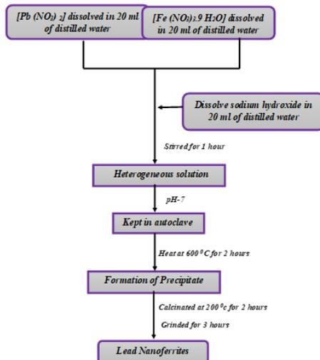
**Figure 2 Flowchart for Lead Ferrite Nanomaterials by Hydrothermal Method**
