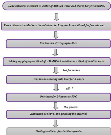
**Figure 1 Flowchart for Lead Nanoferrite Nanomaterials by sol-gel method**
