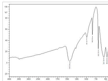
**Figure 7 FTIR spectrum of lead ferrite synthesized by hydrothermal method**
