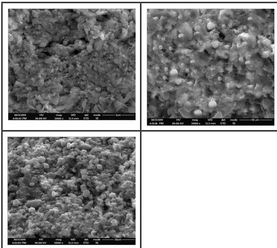
Figure 12 SEM Images of Lead Ferrite made using a Hydrothermal Process
