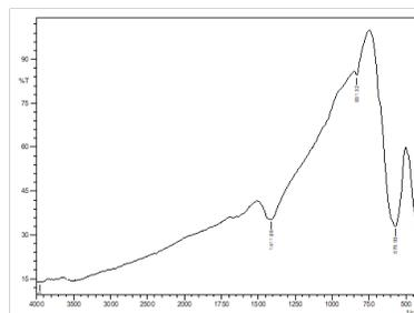
**Figure 6 FTIR Spectrum of Lead Ferrite Synthesized by Sol Gel Method**
