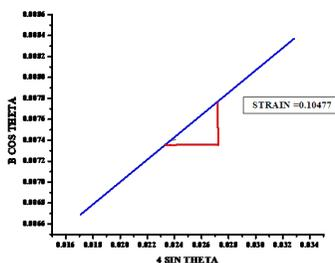
**Figure 5 Williamson's Hall Plot for Lead Ferrite by Sol Gel and Hydrothermal Method**
