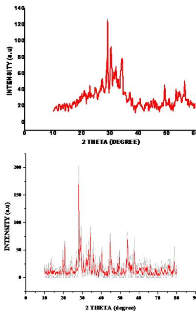
**Figure 4 Lead Ferrite XRD Patterns Produced using the Sol Gel and Hydrothermal Methods**
