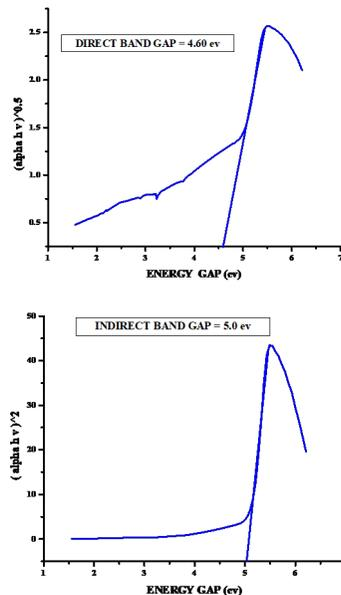
**Figure 10 Direct and Indirect Band Gap for Lead Ferrite by Hydrothermal Method**
