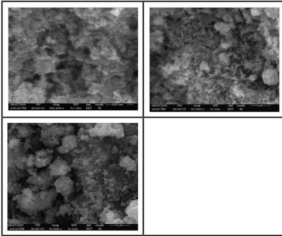
Figure 11 SEM Images of Lead Ferrite Prepared by Sol Gel Method
