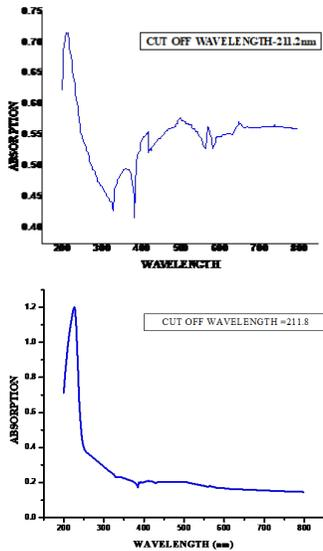
**Figure 8 Cut-off Wavelengths of Lead Ferrite by Sol Gel and Hydrothermal Method**
