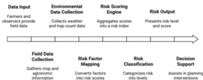
Figure 4 Architecture of the Rule-Based Pest Risk Assessment Model
