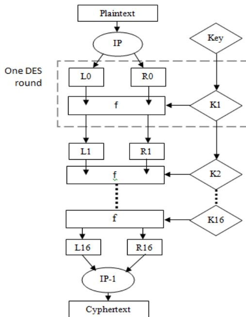
**Fig 1.2: DES Core Algorithm**
